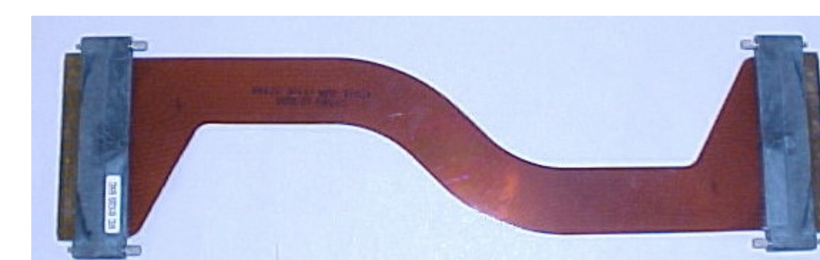
High density pin carriers and flexible kapton transmission lines are key components to the signal feedthroughs. Reviews of Scientific Instruments 76, 063306 (2005)
