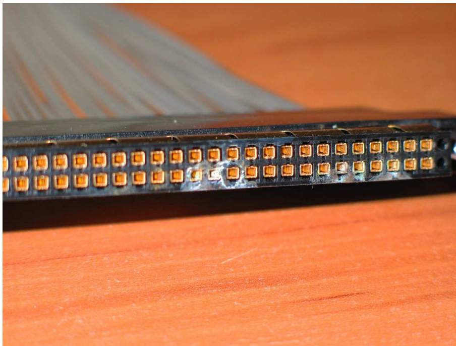
Figure 1: Corroded pin carrier (top) and low voltage warm cable (bottom) from endcap A.
