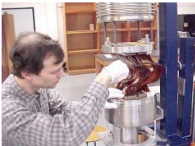
Fig. 2. Vacuum cables being installed on a feedthrough by Paul Birney (TRIUMF) at the University of Victoria.
