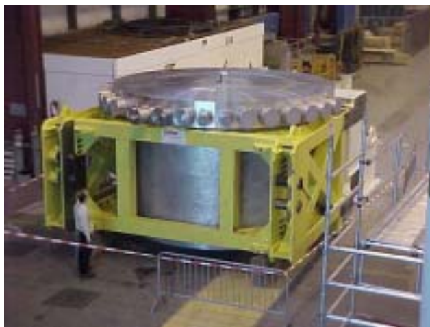
Fig. 3. The first endcap cryostat of the ATLAS liquid argon calorimeter after arrival at CERN, still in its transport cradle (April 2002).
