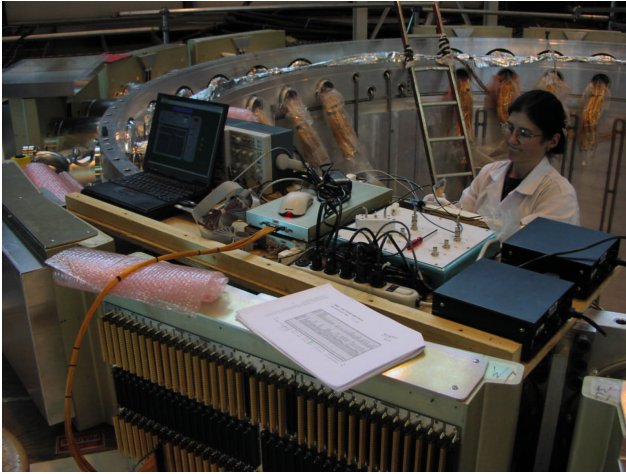
Fig. 6. Fiona Holness (Victoria) performing electrical tests on feedthroughs recently welded on an ATLAS endcap cryostat.
