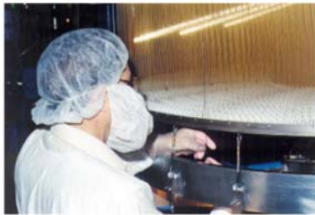
REALLY WIRED: A scientist at TRIUMF, Canada's national laboratory for particle and nuclear physics in Vancouver, replaced 19 of the 29,000 wires in the Canadian-built detector used to probe the nature of anti-matter.
