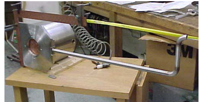
Beam Dump Element being assembled.
