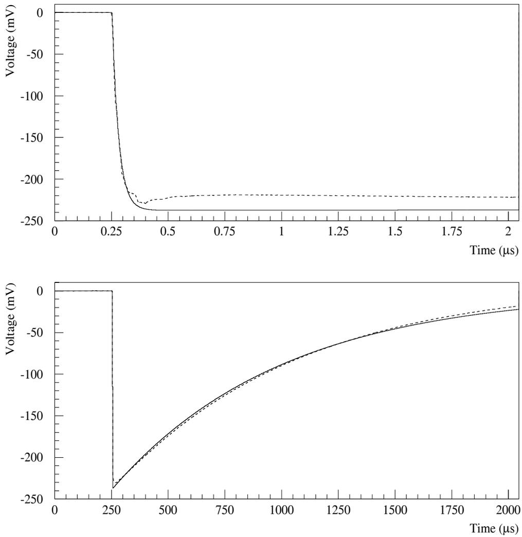
Figure 4.2: Measured ensemble averaged impulse response (dashed line) for the 2.0 mm gap LAr cell, shown with fit (solid line).
