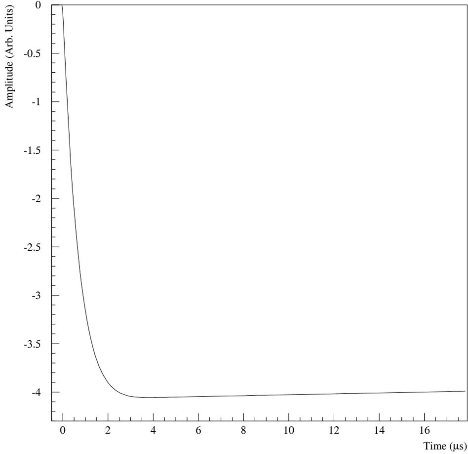
Figure 2.4: A sample theoretical LAr voltage transient of the form given in equation 2.16, with the parameters set to the values obtained in this work.
