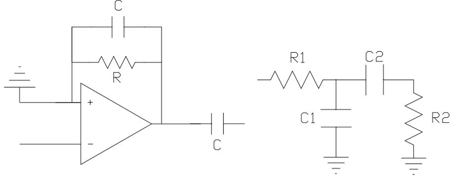
Figure 2.3: Schematic diagram depicting the model used for the preamplifier. The left side depicts the charge integrating preamplifier, which is then modelled as an RC integrator followed by an RC differentiator, as shown on the right.
