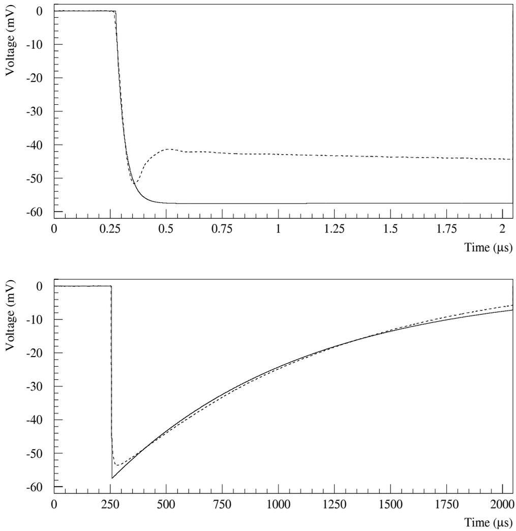
Figure 4.1: Measured ensemble averaged impulse response (dashed line) for the 10.0 mm gap LAr cell, shown with fit (solid line).
