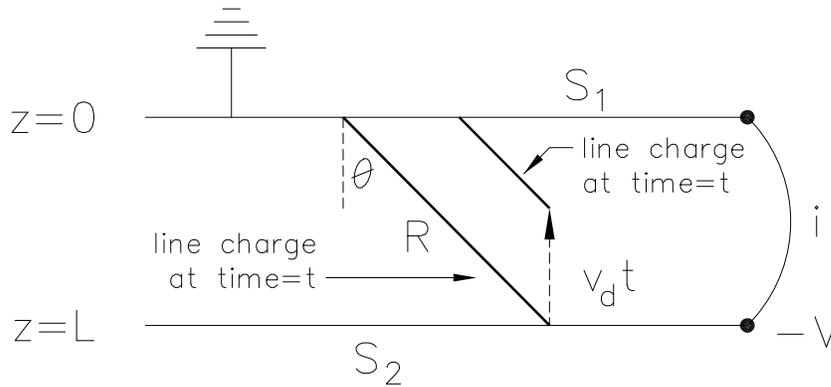
Figure 2.1: Ionization chamber track configuration The line of negative charge of length  $R$  is initially deposited by the passage of the ionizing particle through the cell. At some later time,  $t$ , the line of charge has translated a distance  $v_d t$  upward toward the collection plate located at  $z = 0$ .
