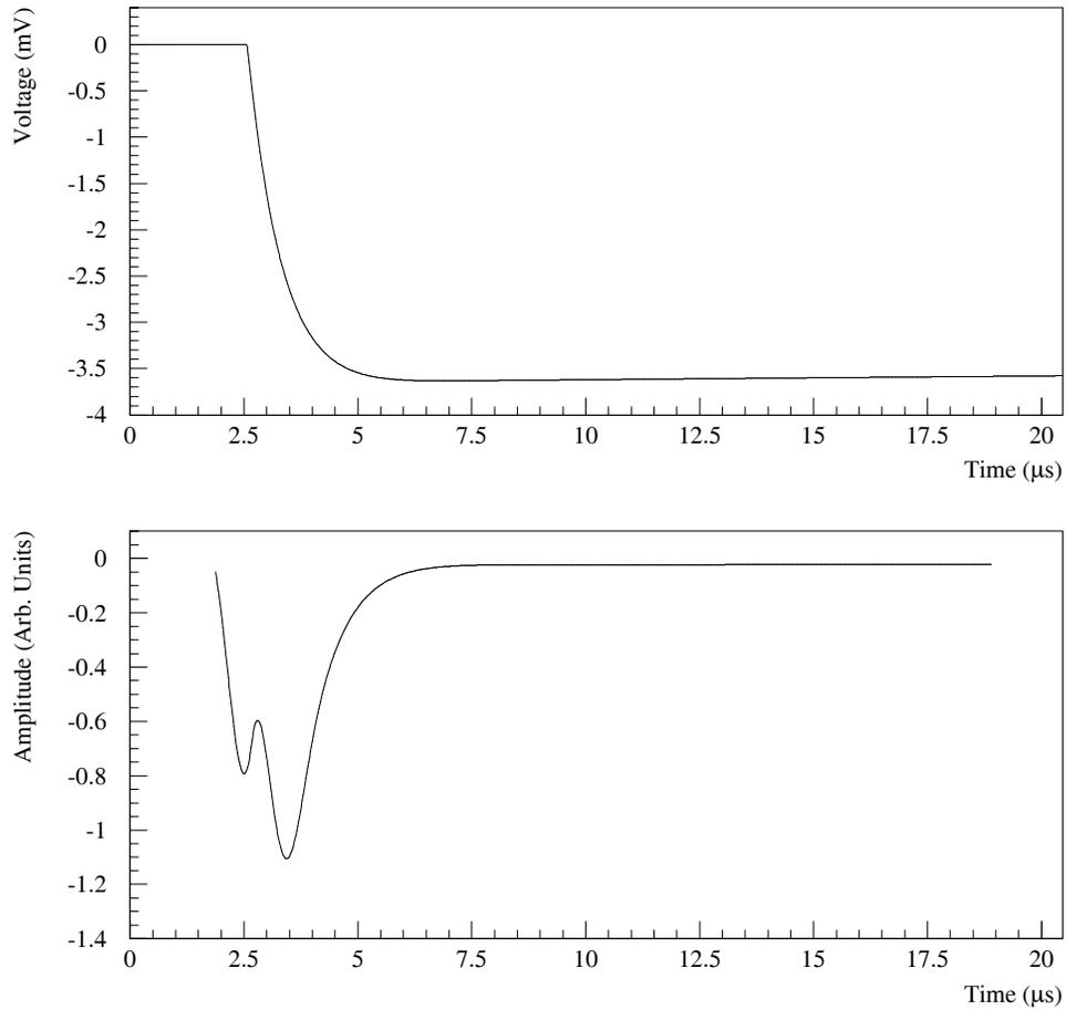
Figure 4.4: A theoretical LAr transient in the top portion of the figure, and its corresponding digitally filtered pulse shown in the lower portion. Notice the absence of data in the leading and trailing regions of the filtered pulse due to initialization and termination of the filtering convolution.
