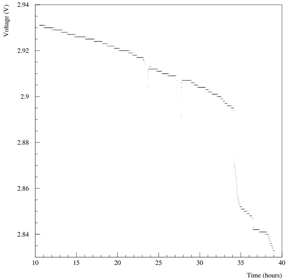
Figure 3.9: Voltage from external  $96.7\Omega$  resistor versus run time of the argon entry. Notice the sharp drop off in the voltage at 34 hours, indicating the internal depth resistor immersing the in the liquid argon. The quantized appearance of the data is a result of the digitization of the CAMAC analog to digital converter.
