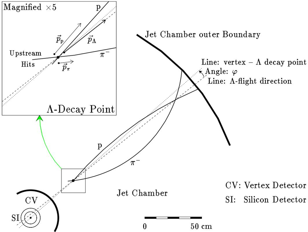
Figure 4.1: Geometry of a  $\Lambda$  Decay in the  $xy$ -Projection Plane
