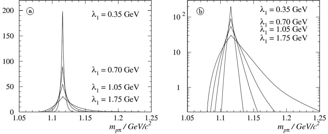
Figure 4.3: Examples of the Fitting Function Used to Describe the  $\Lambda$  Signal In figure (a) a linear scale is chosen while in (b) the same functions are displayed using a logarithmic scale. The parameter  $\lambda_1$  used to calculate an example is written beside the peak of the example function. It can be seen that the function respects the kinematical limits given by  $m = m_p + m_\pi$ . In case of the fit shown in figure 4.2,  $\lambda_1 = 0.42 \text{ GeV}/c$  is found.
