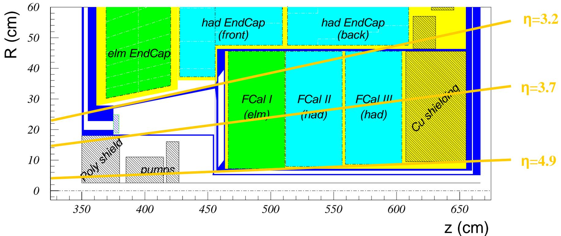
Want to measure calorimeter resolution with and without “simulated” upstream material: cryostat bulkhead, poly shielding, pumps
