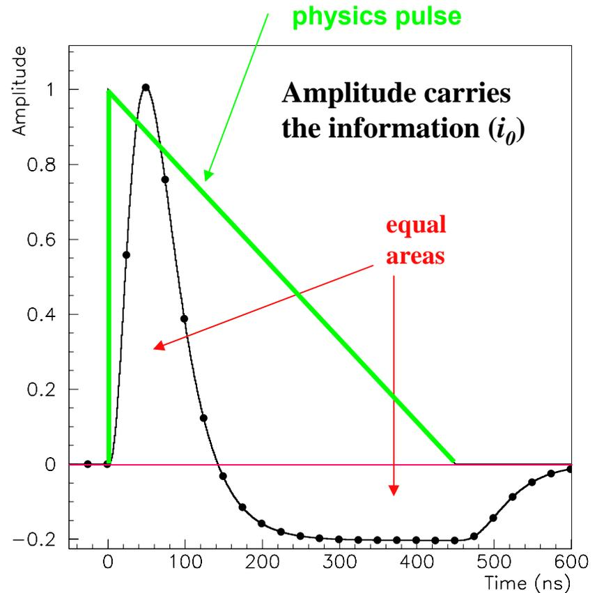
**Optimal shaping time is an optimization problem between electronics noise and pileup noise**
