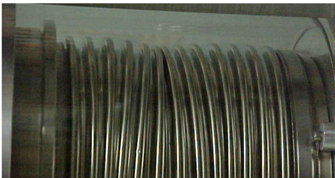
Bellows at 3.5 bar of pressure and no offset.
