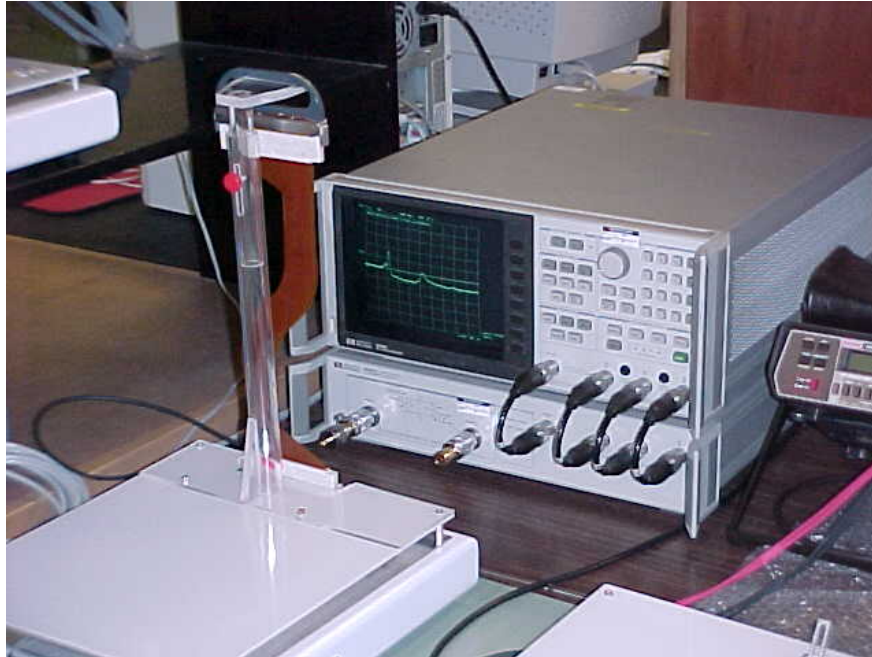
Figure A3 Photograph of the impedance measuring apparatus.
