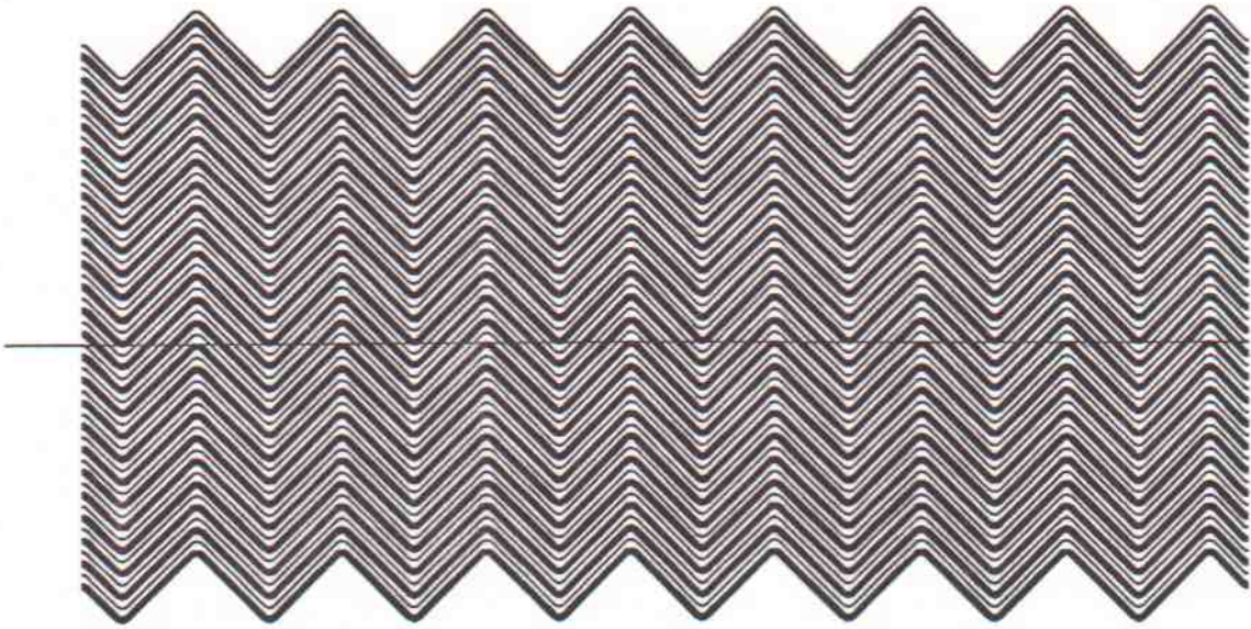
Figure 1: View of the calorimeter in the X - Z plane. The Z axis runs from left to right with Z = 0 at the face. The X axis runs upward. The horizontal line represents a noninteracting particle incident at X = 0 in the fourth readout cell in X . Polar coordinates are defined as usual: \phi is the angle in the XY plane measured clockwise from the X axis and \theta is the angle to the positive Z axis.
