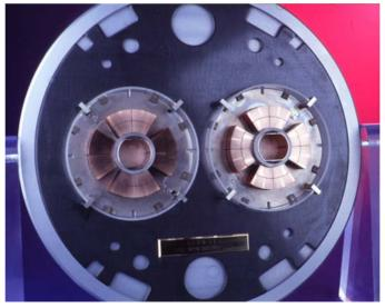
5000 superconducting magnets (1296 dipoles) Cu-clad Nb-Ti cables to operate at 1.9K with up to 15kA
