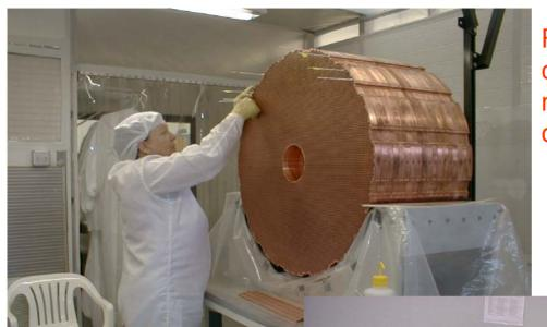
Forward calorimeter module 1 under construction
