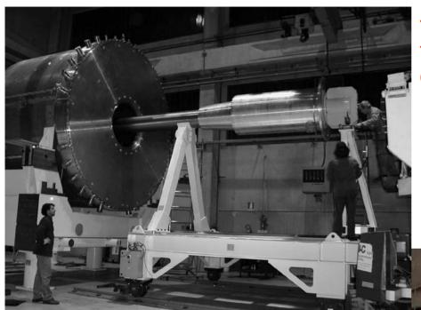
testing the insertion of the FCAL in the endcap cryostat
