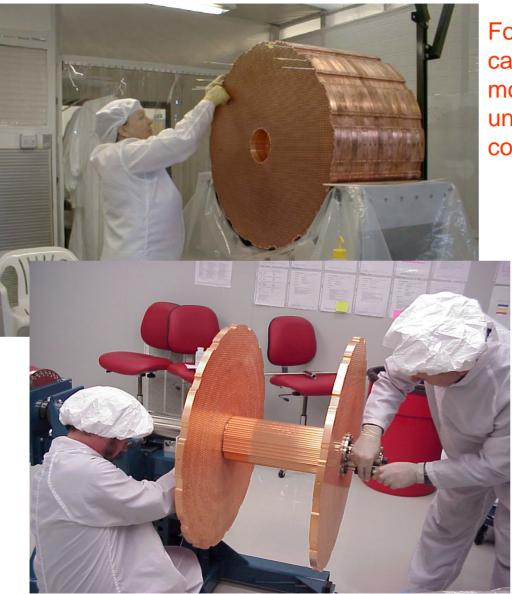
Forward calorimeter module 1 and 2 under construction
