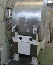
Final touch to a full hadronic endcap inserted into its cryostat
