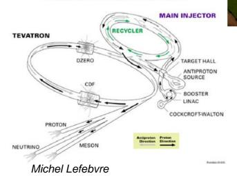
Run I  $\sqrt{s} = 1.8 \text{ TeV}$ 6+6 bunches, 3.5 μs ≈1.6×10<sup>31</sup> cm<sup>-2</sup>s<sup>-1</sup>  $\approx$  2 pb<sup>-1</sup>week<sup>-1</sup> per exp. Run IIa  $\sqrt{s} = 2.0 \text{ TeV}$ 36+36 bunches, 396 ns start March 1st 2001 Now:  $\approx 5 \times 10^{31} \text{ cm}^{-2} \text{s}^{-1}$ > 0.2 fb<sup>-1</sup>per exp. Run IIb  $\sqrt{s} = 2.0 \text{ TeV}$
