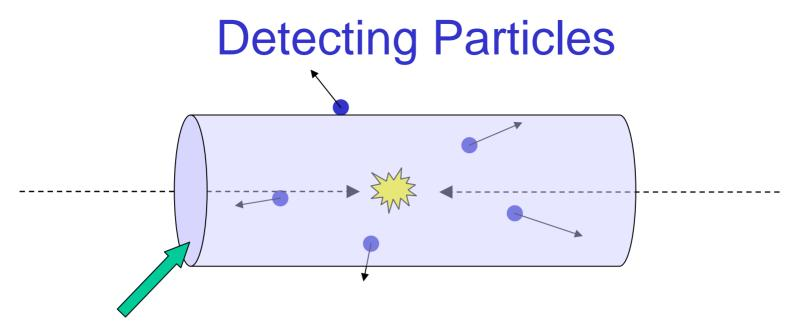
Particle detector: Ideally, identify, for each particle produce in each collision, its type (mass, electrical charge, spin, other quantum numbers), and its 4-vector (energy, px, py, pz) at the interaction point.
