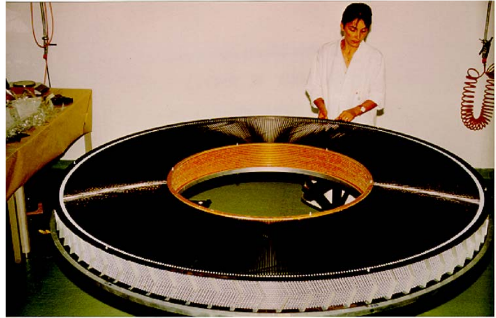
ATLAS Transition radiation Tracker using about 400 000 straw tubes detectors with Xe based gas
