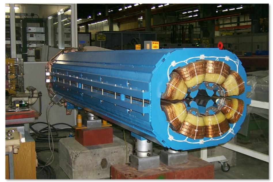
48 + 4 warm twin-aperture quadrupoles for cleaning insertions
