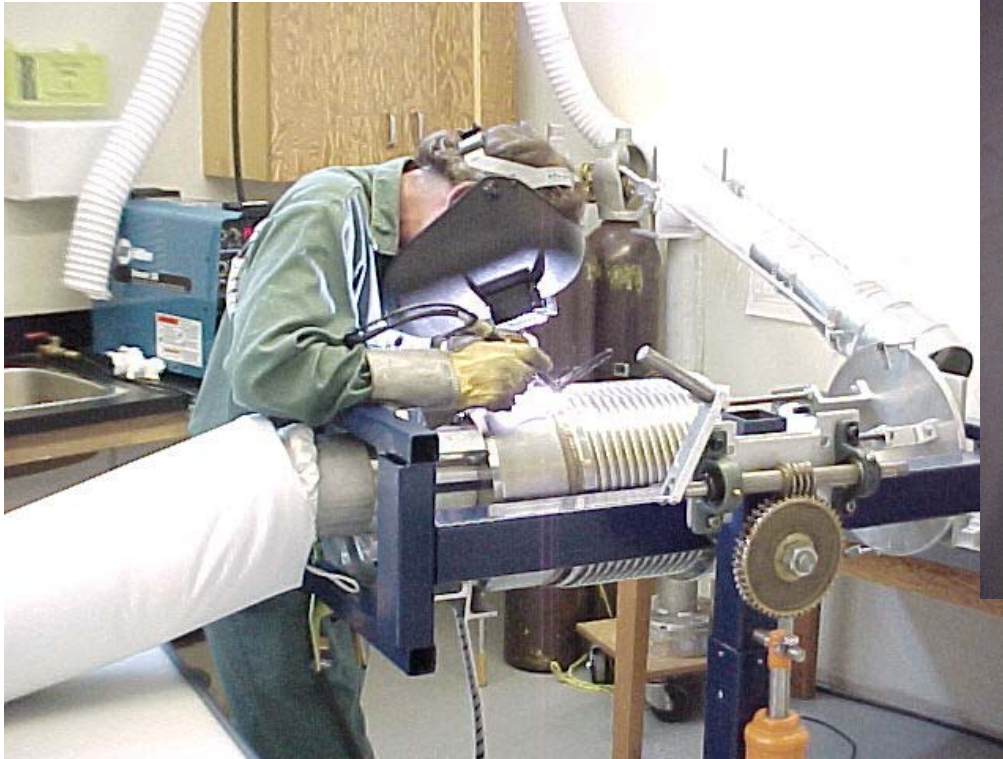
welding of feedthrough
