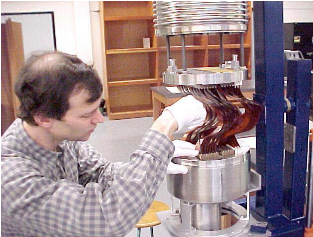
vacuum cable installation
