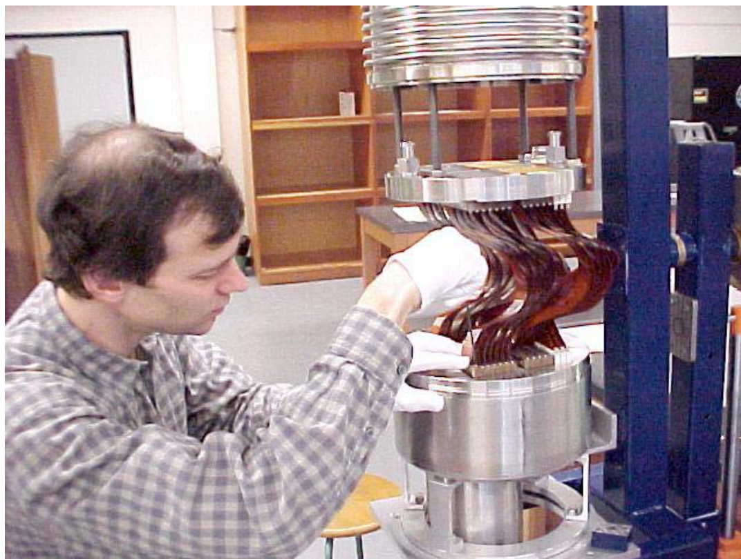
vacuum cable installation
