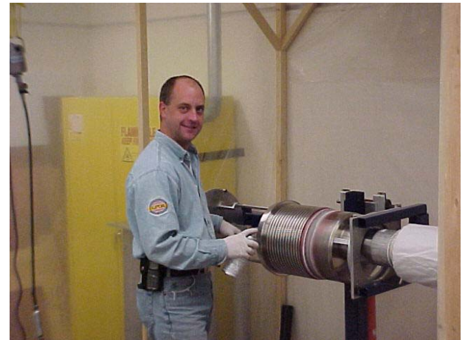
last dye penetrant tests
