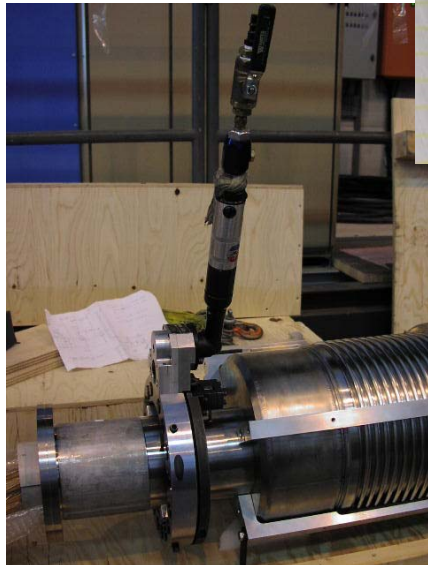
weld with orbital welder
