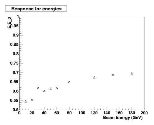
• The energy response shows a non-linear dependence on the pion beam energy, as expected for a non-compensating calorimeter
