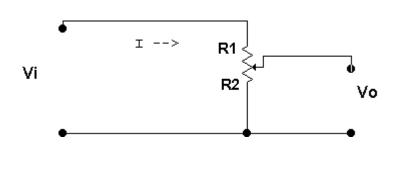
$R = R_1 + R_2$  is fixed position of wiper sets  $R_1$  and  $R_2$ :
