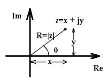
The modulus can be associated with, for example, the peak voltage of a waveform and  $\theta$  as the relative phase of the waveform.
