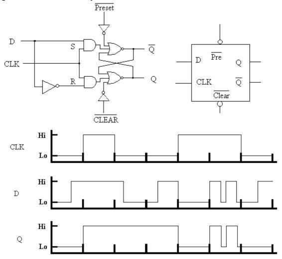
This is still a transparent latch. But, the logic race condition can be avoided again by using edge triggering, either rising or falling edge. In the lab, you'll be using a 7474 Dual D-type Flip-flop.i.e. Two FF in one IC package.
