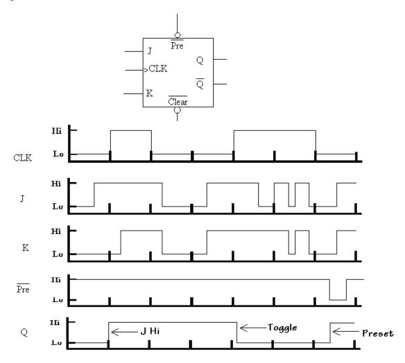
In the lab you'll use a falling-edge CLK (7476 JK-FF) so that, unlike in the above example, the inputs are examined only when the CLK transition goes from Hi to Lo. It also has active low PRESET and CLEAR.
