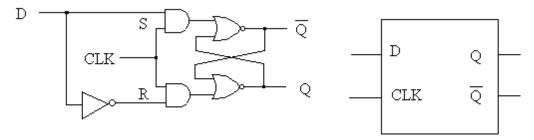
In this way the undefined states can be avoided altogether. Then there is only one input, S, which is renamed D, for data. When D is Hi when the CLK is Hi, then Q goes Hi. When D is Lo when the CLK is Hi, then Q goes Lo.
