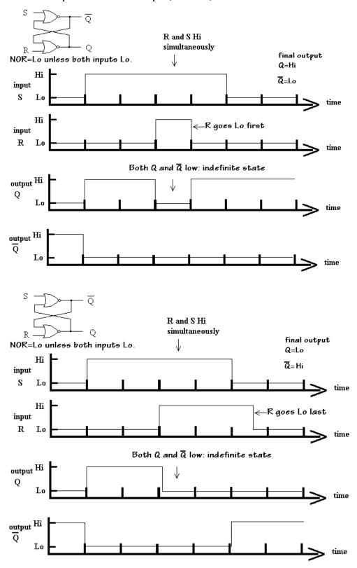
This is clearly not good. There are several ways of dealing with this problem. A simple way is to only allow a Set or Reset when a third signal allows it.
