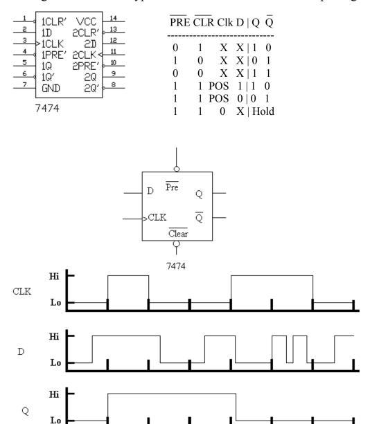
The D-type flip-flop is one specialized configuration of the RS flip-flop designed to remove the undefined status. It is a standard memory element that can be written to synchronous with the clock or cleared/set asynchronously.
