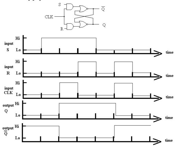
When the CLOCK is Lo, the data is said to be *latched* which means the system is disabled for new data. We can only 'write into memory' when the CLOCK is Hi.
