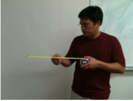
Figure 23: The tape measure blade shown just before buckling.
