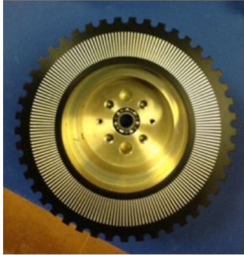
Figure 16: The optical encoder wheel engraved on underside of boom reel.
