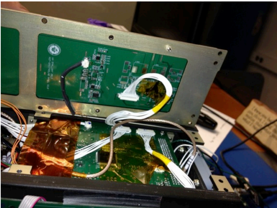
Figure 27: Attaching the x-axis solar panel to H2 during final assembly.
