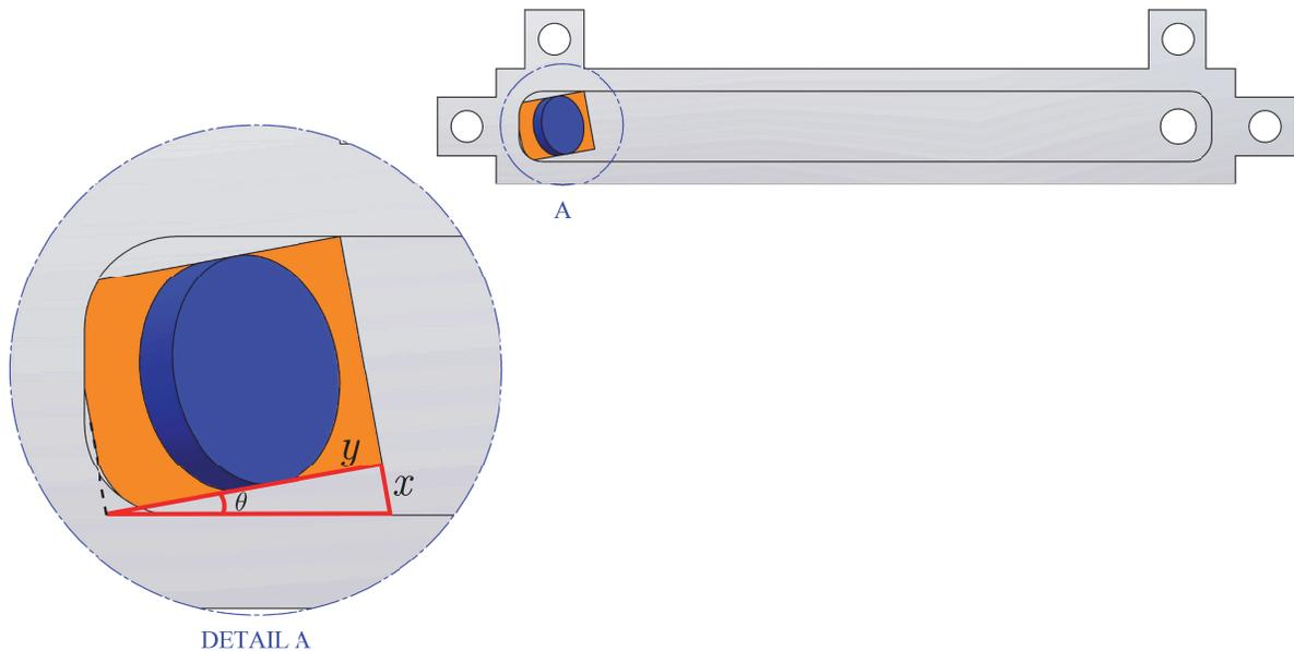
Figure A.5: Alignment of small mirrors in the optical path module suffers from the 5 thou machining error.
