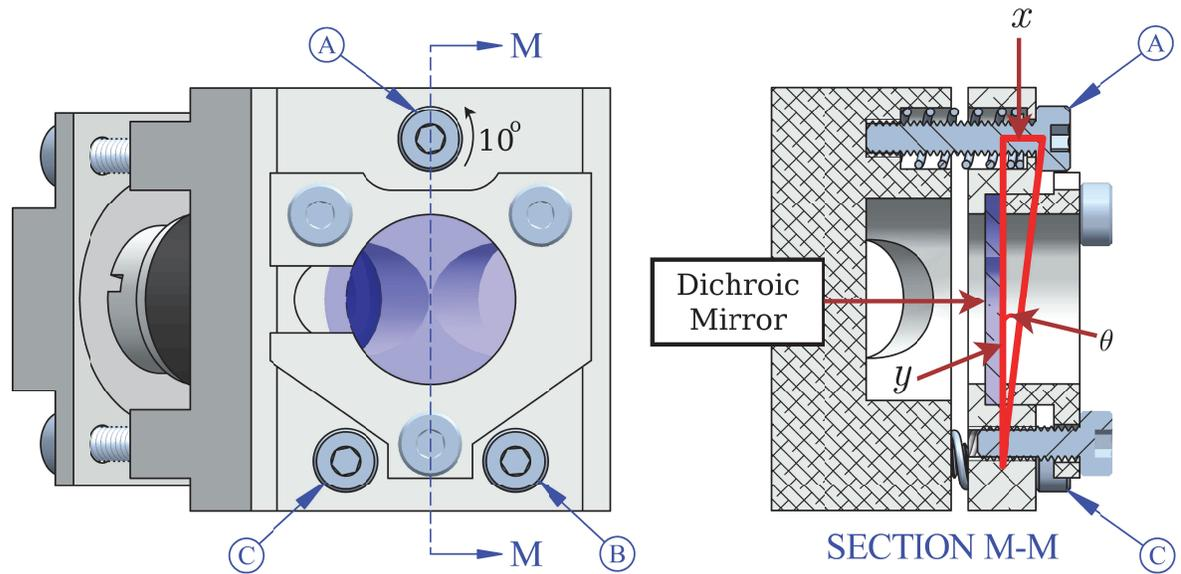
Figure A.3: Dichroic mirror's spring-loaded surface-angle adjustment mechanism. Rotating each of the screws A, B or C changes the angle of dichroic mirror's surface with respect to the incident laser beam.
