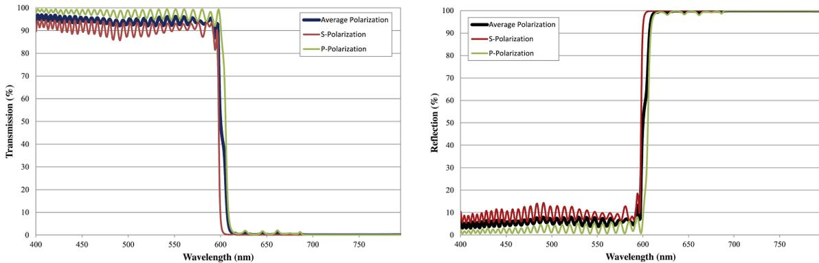
(b) Graphs of a DM2 - a shortpass dichroic mirror with cut-off wavelength of 600 nm. Right: transmission graph; left: reflection graph [31].
