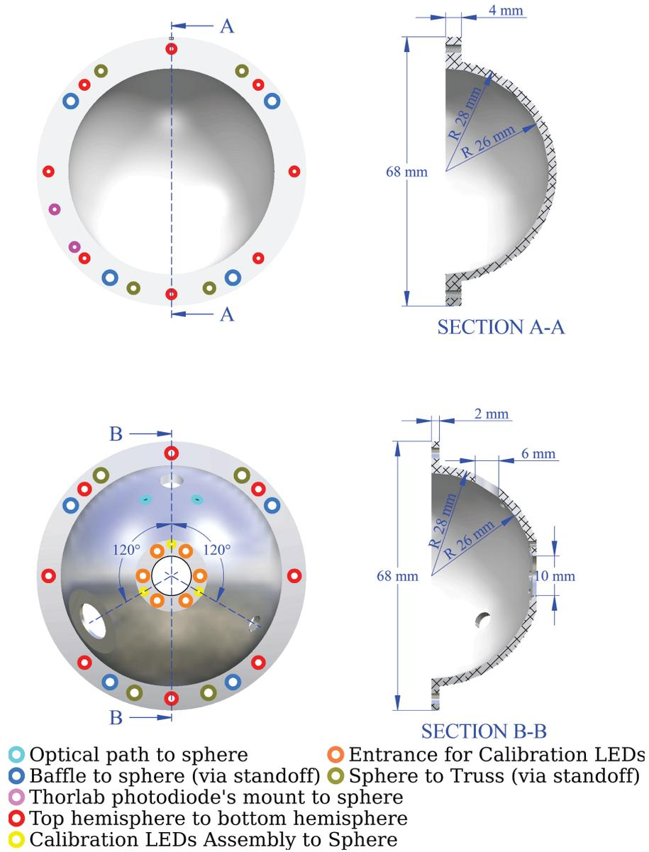
Figure A.1: Engineering drawing of the integrating sphere designed at SFL.
