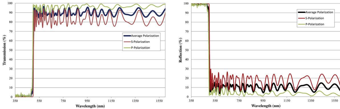
(a) Graphs of DM1 - a longpass dichroic mirror with cut-on wavelength of 500 nm. Right: transmission graph; left: reflection graph [30].
