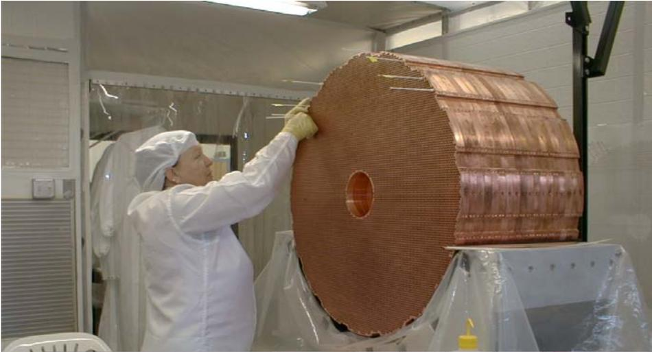
Forward calorimeter module 1 and 2 under construction
