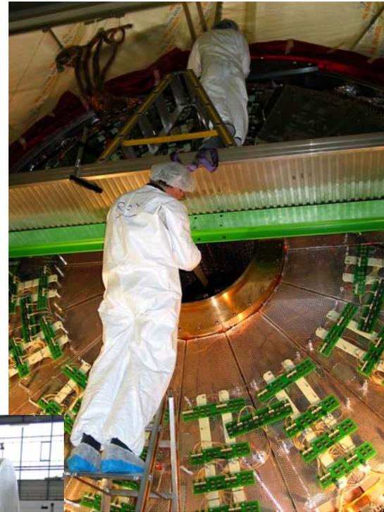
Final touch to a full hadronic endcap inserted into its cryostat
