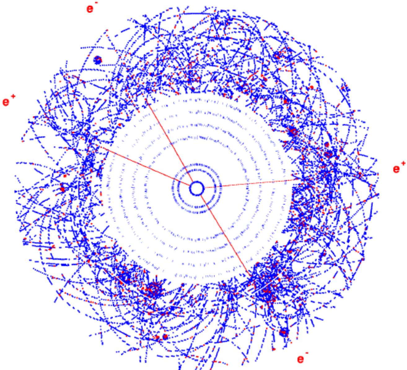
High luminosity simulation. Precision hits are shown for  $0 < \eta < 0.7$ ; TRT hits are shown in barrel for  $z > 0$ ; high threshold transition radiation hits are shown as red points. Fitted tracks (red), with  $p_T > 5$  GeV and  $0 < \eta < 0.7$ , are shown just in the precision tracker so as not to obscure the TRT hits.
