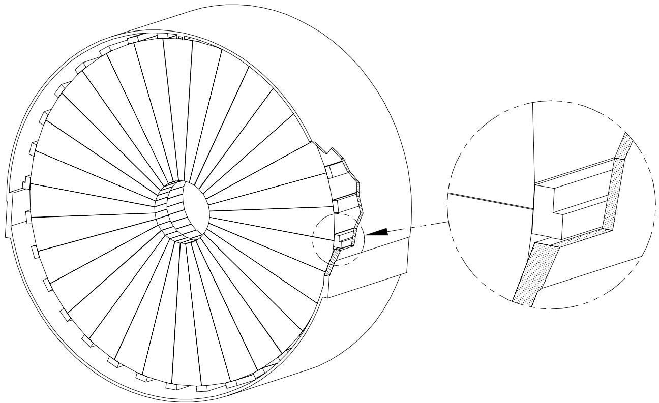
**Composed of 2 wheels per end, 32 modules per wheel**
