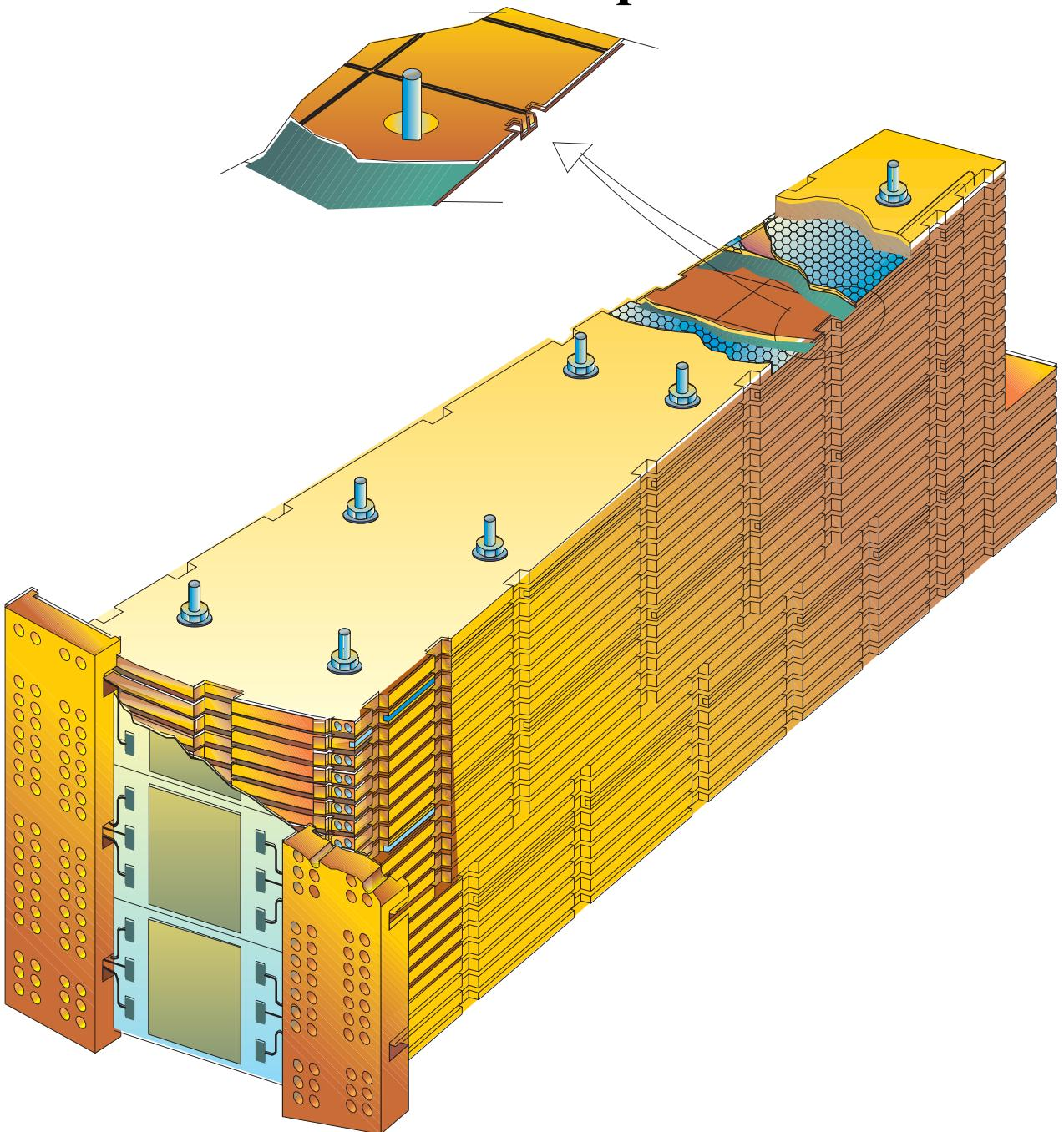
**Gap between Cu plates:** **8.5 mm**
