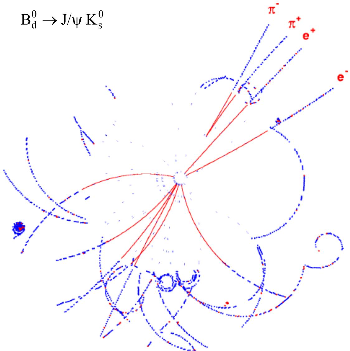
Low luminosity simulation. Precision hits are shown for  $0 < \eta < 0.7$ ; TRT hits are shown in barrel for  $z > 0$ ; high threshold transition radiation hits are shown as red points. Fitted tracks (red), with  $p_T > 0.5 \text{ GeV}$  and  $0 < \eta < 0.7$ , are shown just in the precision tracker so as not to obscure the TRT hits.
