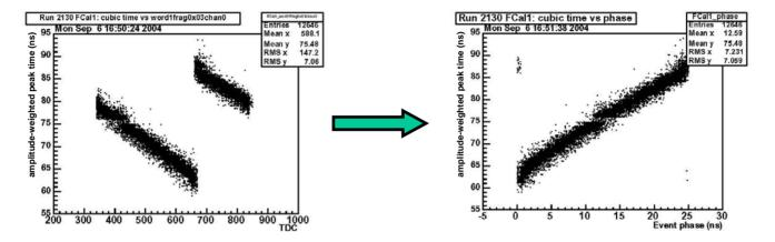
The goal of TBPhaseRec is to produce a phase (0.0 to 25.0 ns) related to the event time as in the right figure, given at least one raw TDC value, as in the left figure.
